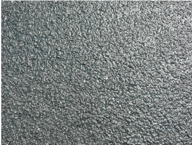
Fig. 1 Test C - Slip resistance - surface type – Grit Grade 16 (Industrial/Coarse)
